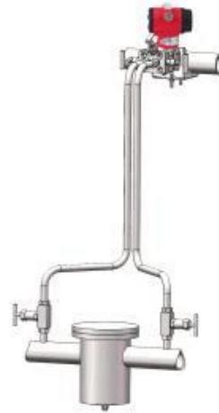
Pipe Differential Pressure Measurement
