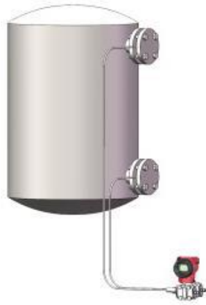
Tank Liquid Level Measurement
